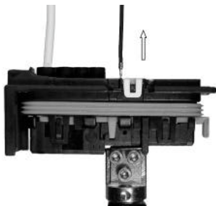
Fig. 16: 26-way contact housing, removal of BMK 0.6 terminal
