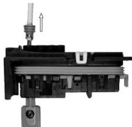
Fig. 17: 26-way contact housing, removal of MCP 2.8 terminal
