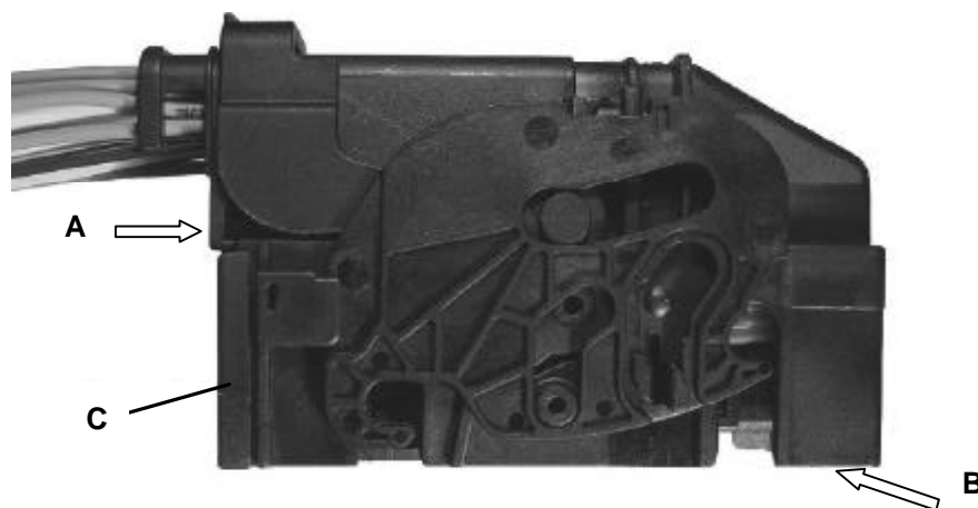
Fig. 22: Releasing the catch holding the contact housing in the cover
